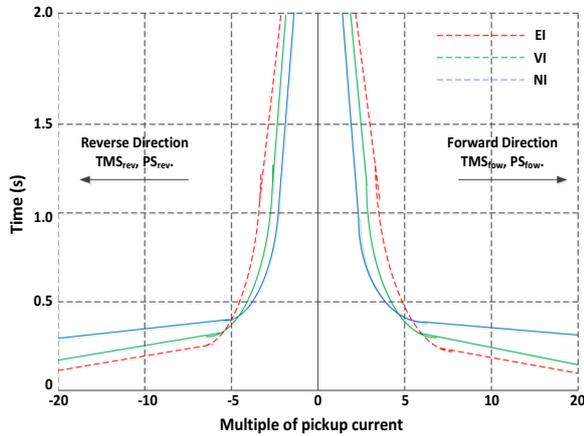
Fig. 1 Time-current characteristics of a dual setting DOCR
