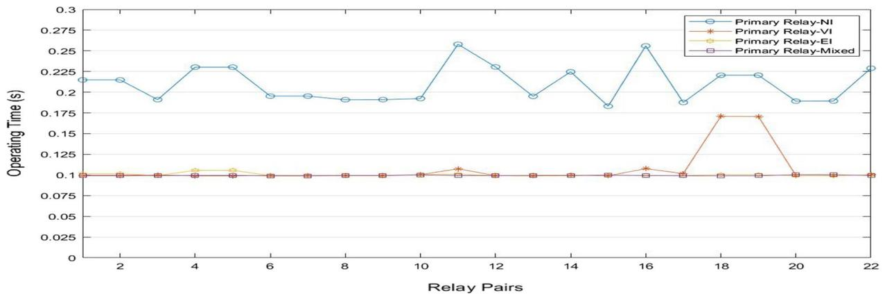
Fig. 5 Primary relay operating time having NI, VI, EI and mixed characteristics in grid-connected mode
