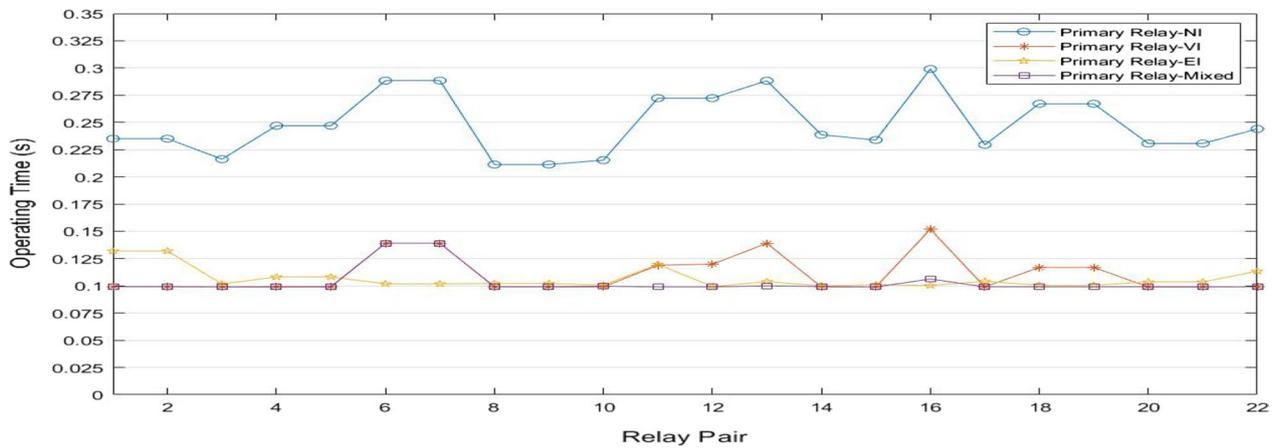
Fig. 8 Primary relay operating time having NI, VI, EI and mixed characteristics in islanded mode
