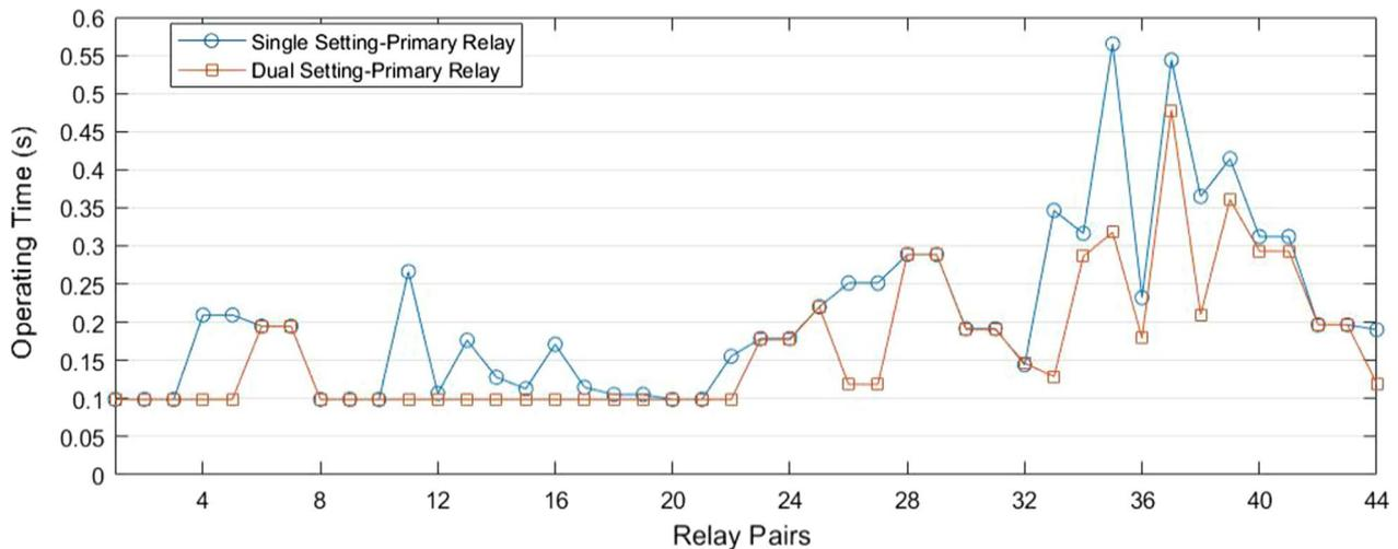
**Fig. 10** Primary relay operating time using single and dual setting DOCR for common relay setting
