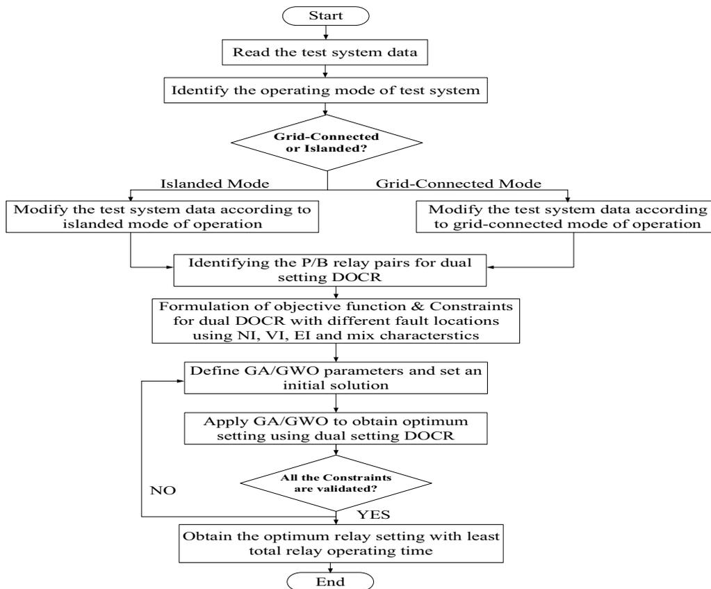
**Fig. 3** Proposed protection method to determine optimal relay setting in grid connected and islanded operating mode
