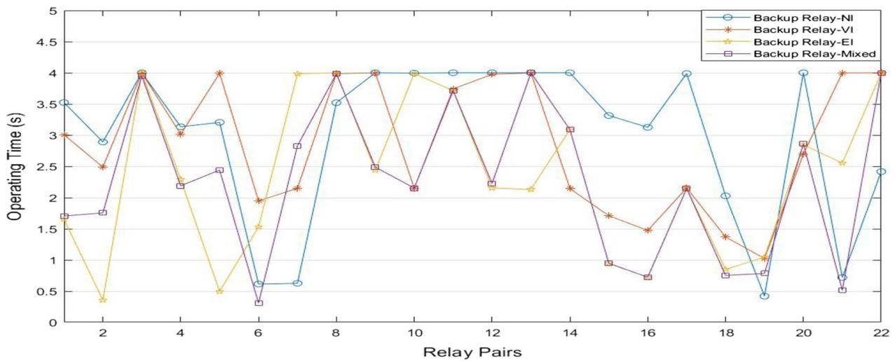
Fig. 7 Backup relay operating time having NI, VI, EI and mixed characteristics in grid-connected mode
