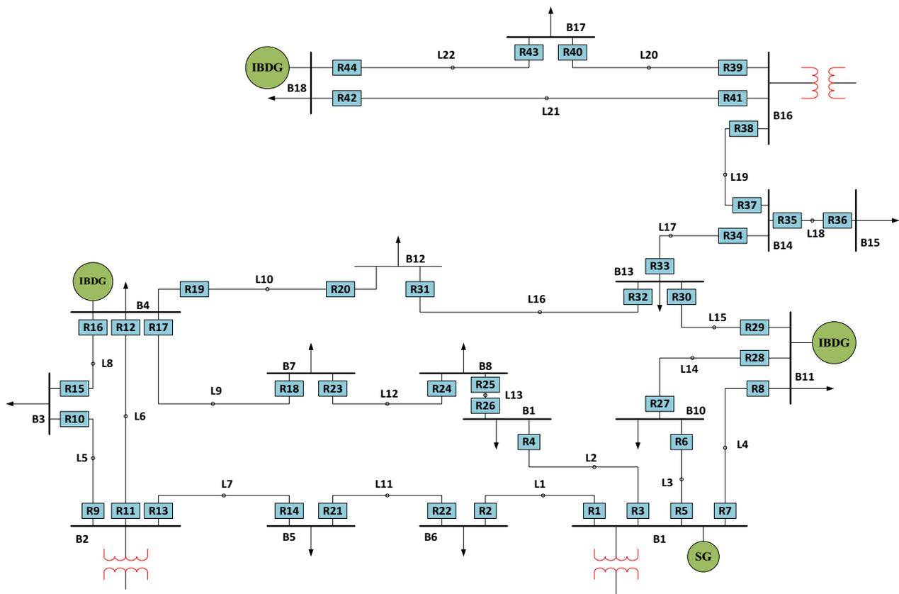
**Fig. 11** Distribution part of IEEE-30 bus system (18-bus microgrid system)
