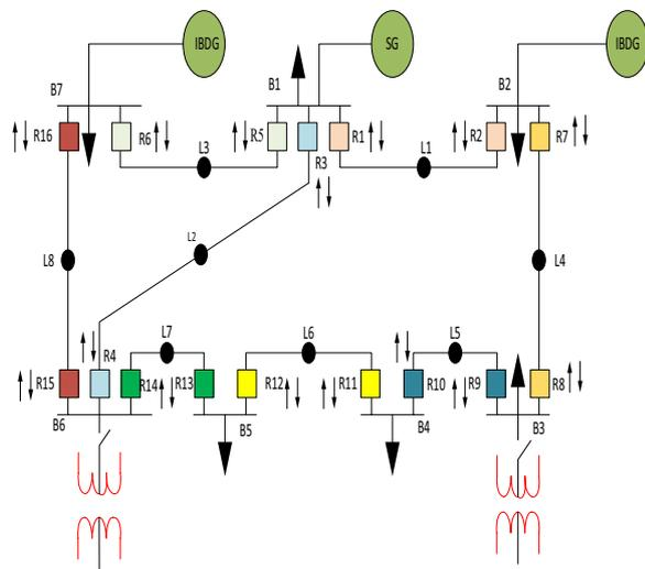
**Fig. 4** Distribution part of IEEE-14 bus test system with dual setting DOCR
