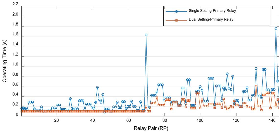
**Fig.12** Primary relay operating time using single and dual setting overcurrent relays for common relay setting in 18 bus microgrid test system
