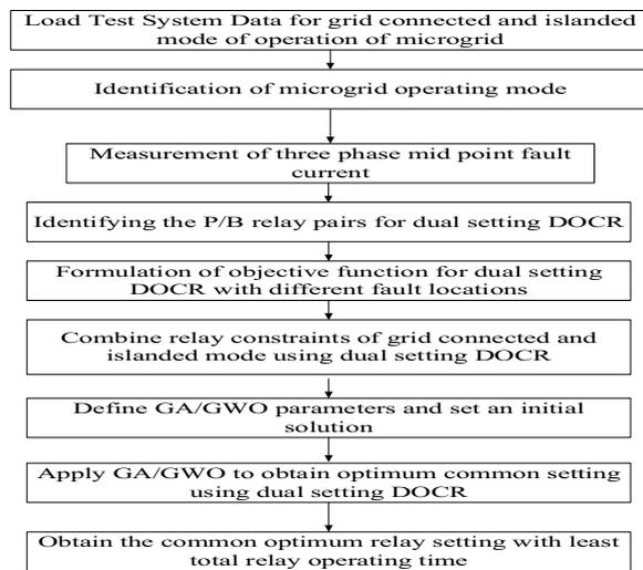
**Fig. 9** Method for common optimal setting for dual operating modes of MG
