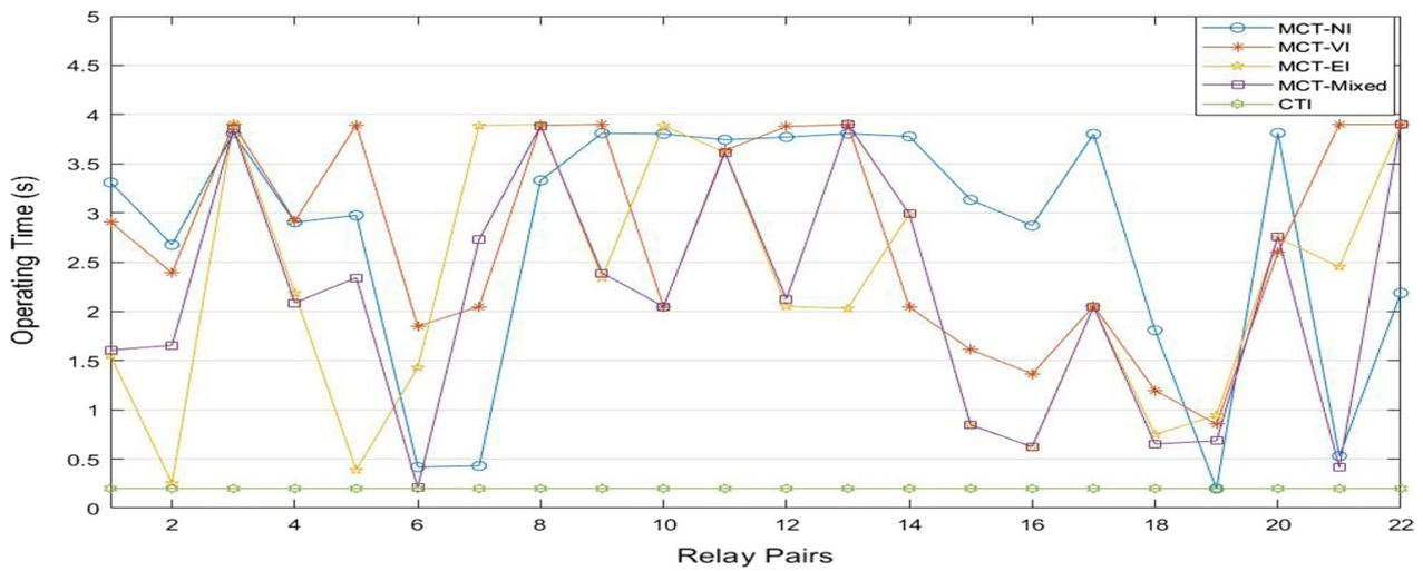
Fig. 6 MCT having NI, VI, and EI and mixed characteristics using dual setting DOCR in grid-connected mode
