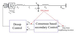
**Fig. 8** Illustrative diagram of consensus-based control of inverter *i* under FDI attacks
