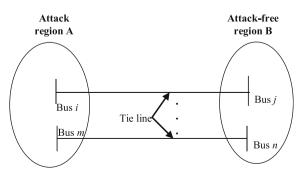
**Fig. 5** A power system decomposed into attack and attack-free regions
