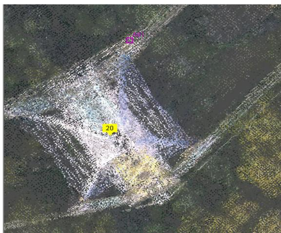
**Fig. 5** A recognized transmission tower. The yellow point represents the transmission tower recognized by the proposed method
