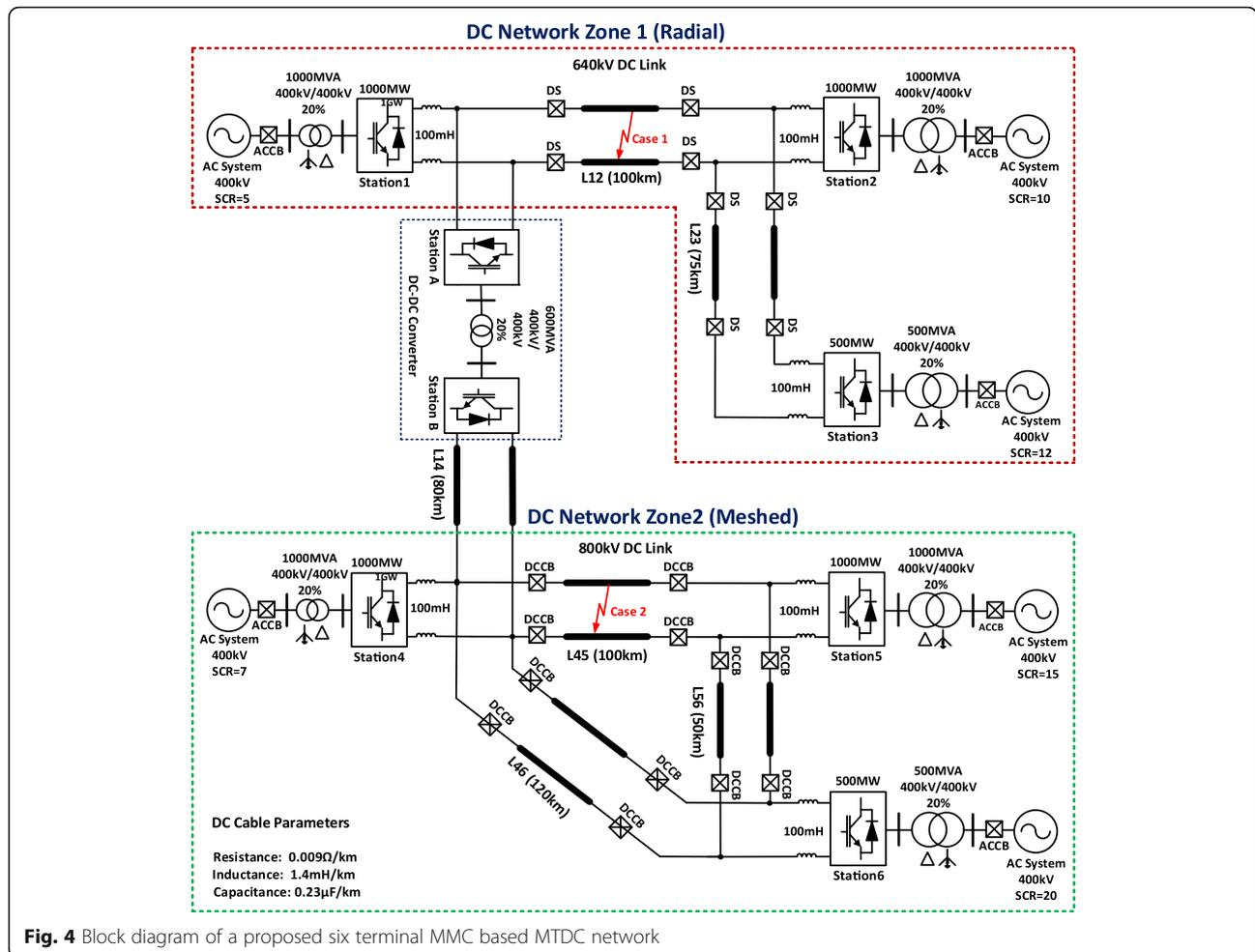
Fig. 4 Block diagram of a proposed six terminal MMC based MTDC network
