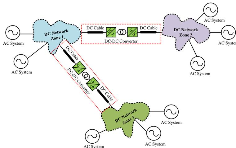
**Fig. 3** Possible partitioned MTDC networks using DC-DC converters
