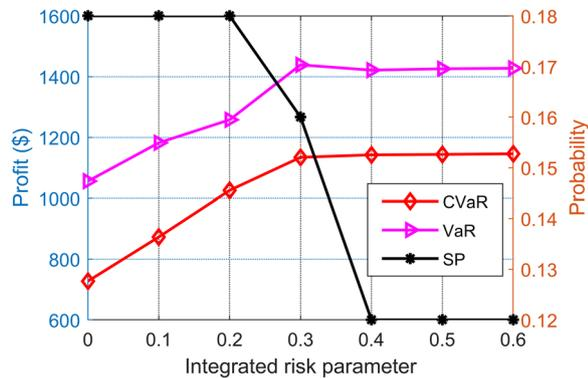
**Fig. 6** The risk measurement results of wind storage system with different integrated risk parameters
