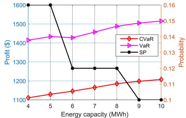
**Fig. 8** The risk measurement results of a wind storage system with different storage energy capacities
