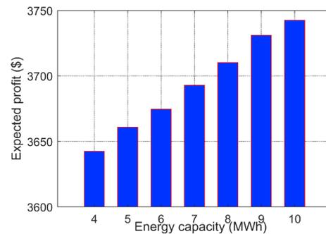
**Fig. 9** The expected profits of a wind storage system with different storage energy capacities
