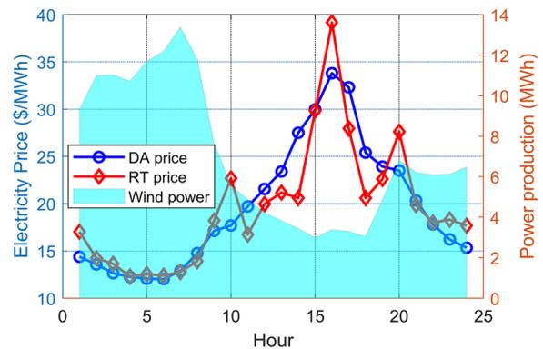
Fig. 3 The expected values of day-ahead and real-time electricity prices and wind power productions
