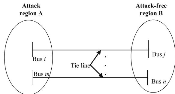
Fig. 5 A power system decomposed into attack and attack-free regions
