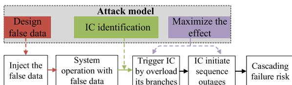
Fig. 3 Illustration of cascading failures caused by FDI [3]
