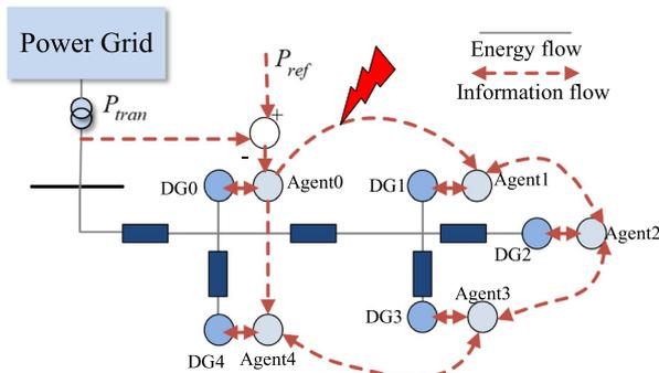
**Fig. 7** Illustrative diagram of distributed control of distributed generators
