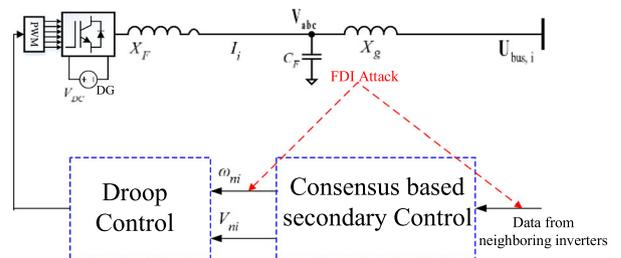
**Fig. 8** Illustrative diagram of consensus-based control of inverter  $i$  under FDI attacks
