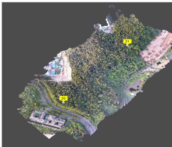
**Fig. 4** A photograph with transmission towers. The yellow points represent transmission towers in this tilt photography photo of transmission line with fixed-wing UAV
