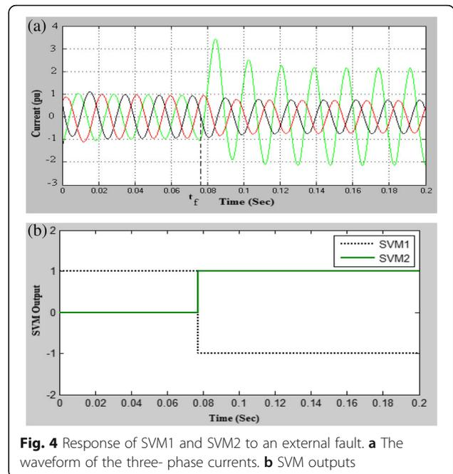
**Fig. 4** Response of SVM1 and SVM2 to an external fault. **a** The waveform of the three-phase currents. **b** SVM outputs
