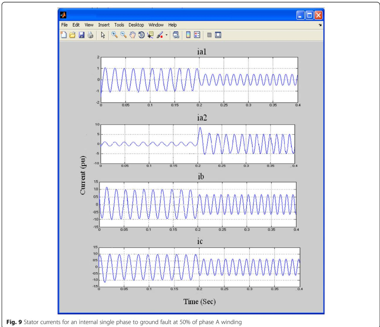
**Fig. 9** Stator currents for an internal single phase to ground fault at 50% of phase A winding
