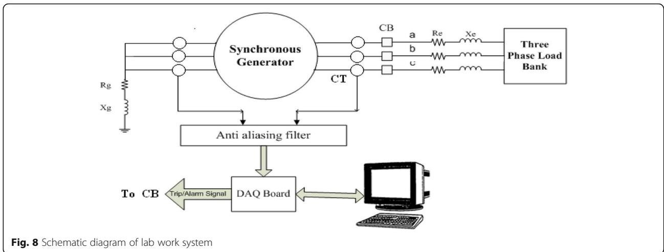
**Fig. 8** Schematic diagram of lab work system
