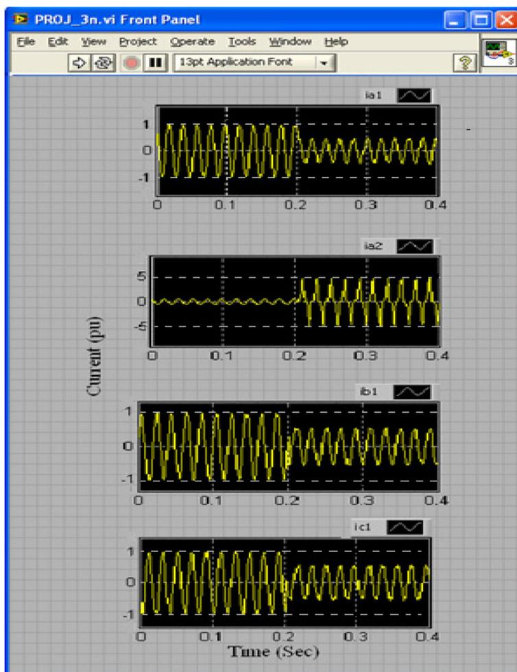
**Fig. 10** Recorded stator currents for an internal single phase to ground fault at 50% of phase A winding
