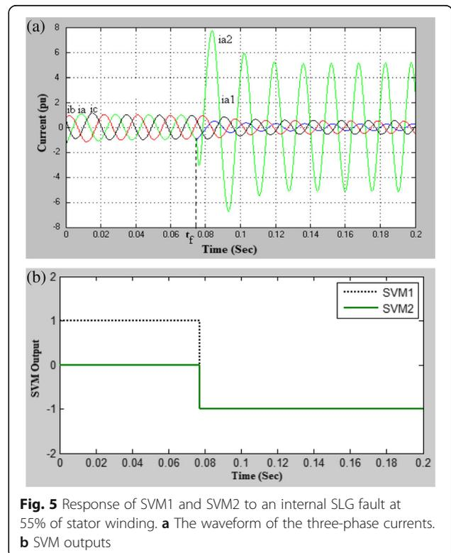
**Fig. 5** Response of SVM1 and SVM2 to an internal SLG fault at 55% of stator winding. **a** The waveform of the three-phase currents. **b** SVM outputs
