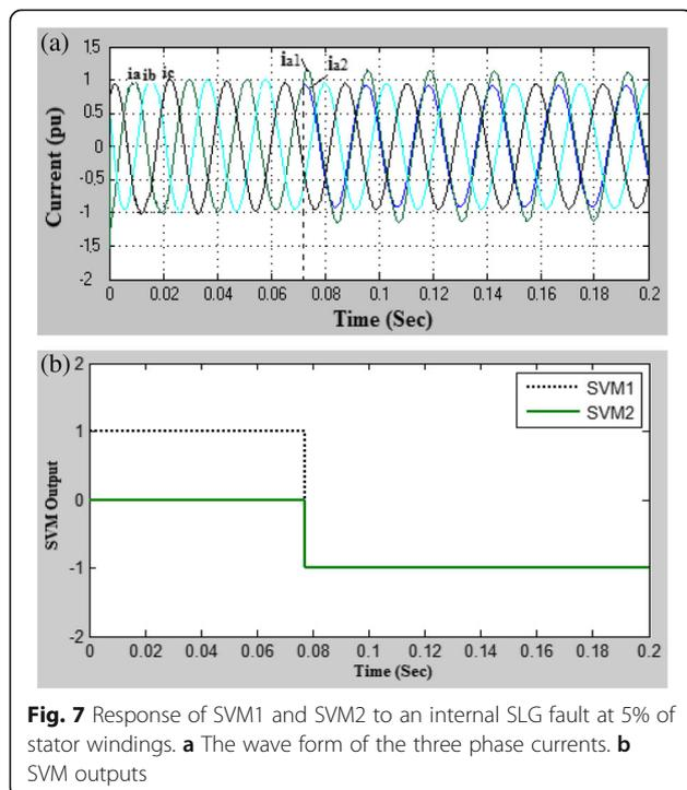
outputs under normal steady state conditions and rapid convergence of the output variables to the expected values under fault conditions. This clearly confirms the effectiveness of the proposed SVM based fault detector.
