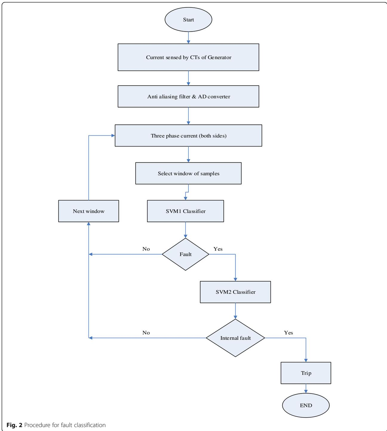
SVM1 represents a normal state, its output is set to +1; otherwise it is set to - 1. On other hand, SVM2 is trained to discriminate between internal fault state and external fault state. Its output will be +1 for input patterns representing internal faults and -1 otherwise.
