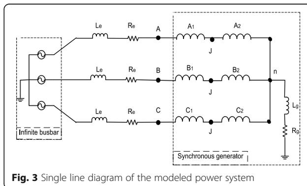
**Fig. 3** Single line diagram of the modeled power system
