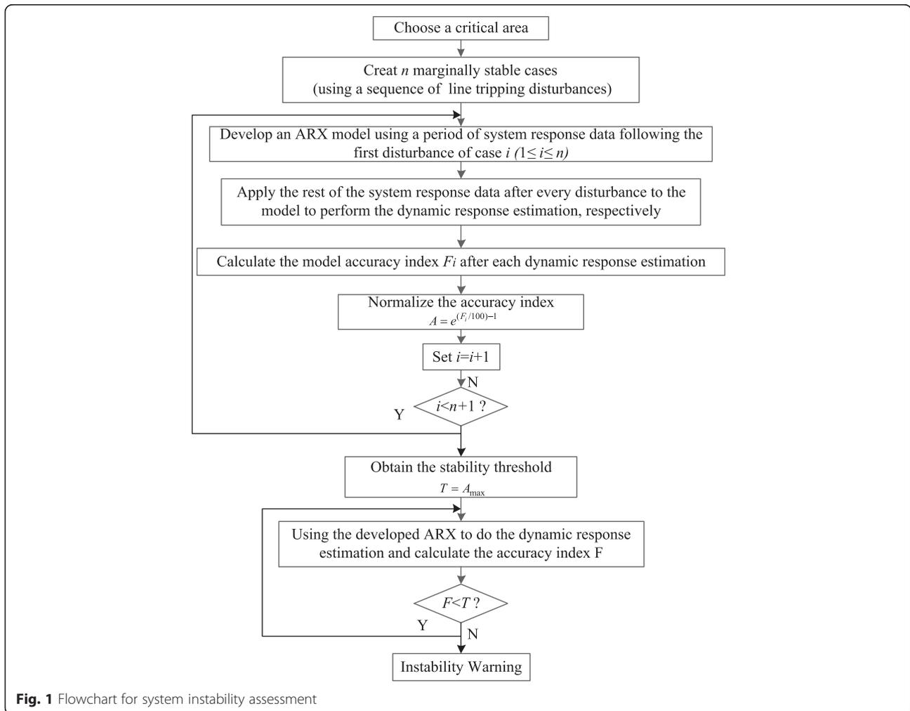
**Fig. 1** Flowchart for system instability assessment
