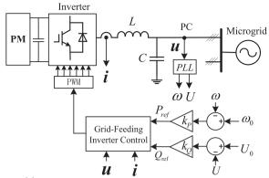
(a) Control block diagram of PQ-droop grid-supporting inverter
