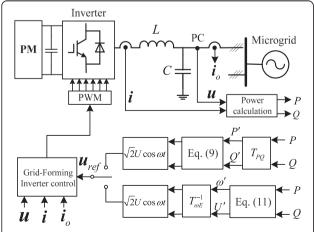
**Fig. 7** Control block diagram of ωU-droop Grid-supporting inverter applying decoupling transformation method
