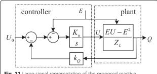
**Fig. 11** Large-signal representation of the proposed reactive power control
