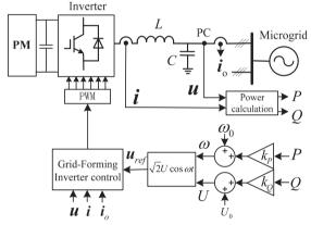
(b) Control block diagram of ωU-droop grid-supporting inverter
