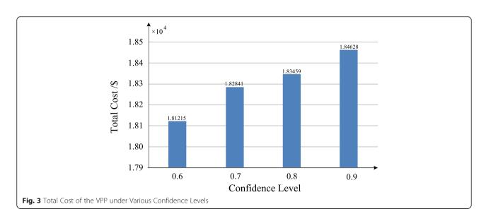
risk tolerance of VPPs. Further, through transforming the fuzzy chance constraints into their equivalent forms, the conventional optimization algorithms can be utilized to solve the optimal scheduling problem. The case study proves that the operational cost of VPPs will increase when the confidence level increases. That is to say, unnecessary costs can be reduced when the risk of VPP operation is within tolerance.
