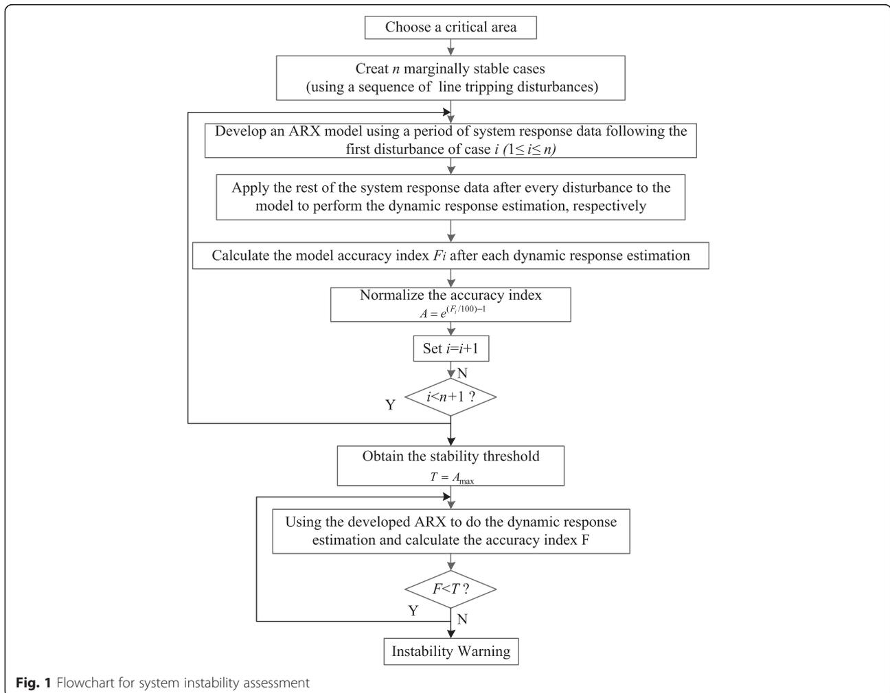
**Fig. 1** Flowchart for system instability assessment
