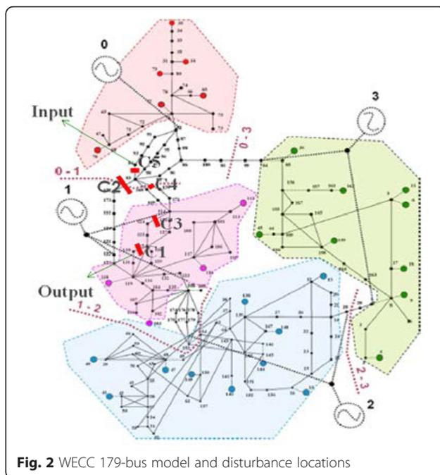
**Fig. 2** WECC 179-bus model and disturbance locations
